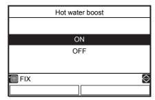
When the set time period has passed or the water temperature has reached the set temperature, the hot water boost operation ends automatically.
