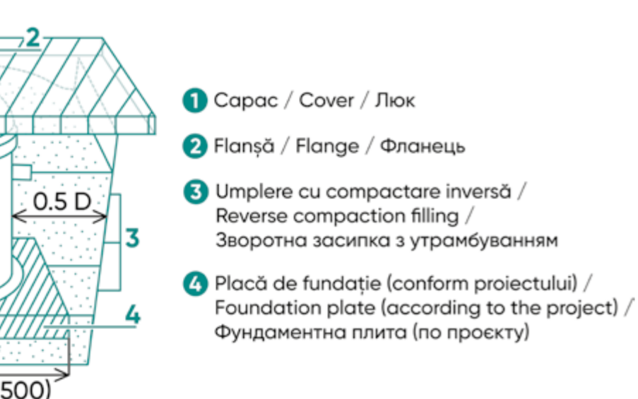
Fig.5 Schematic diagram of the installation of a vertical enclosure in the high groundwater level 2 area in a pedestrian area
